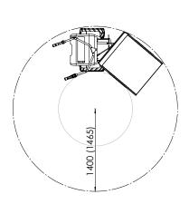
All dimensions unless otherwise stated are in millimetres. Dimensions B300 BENDie (B450 BENDie)
